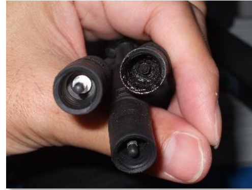
DC connectors arcing poor connection
