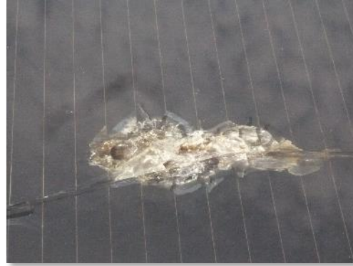
Cracked PV module glass over heating Junction box
