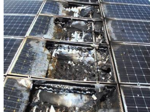
PV string fire due to DC arcing
