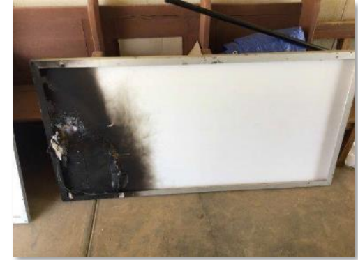
Module Junction box and hot spot DC arcing
